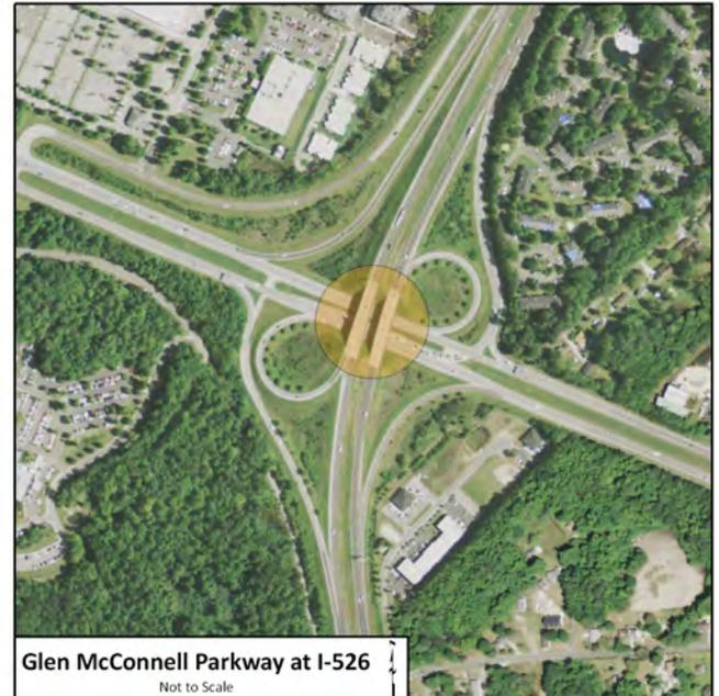
The preferred interchange layout is chosen to be Hybrid Single Point Urban Interchange (SPUI) with a single directional flyover ramp due to less significant impact to the surrounding area in terms of Right-of-Way requirements, environment impacts, access constraints, and merge/weave conflicts.
